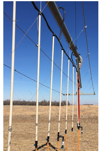
(Above) HLDCM - Showing overhang cable supports. (See page 10 Figure 1)
