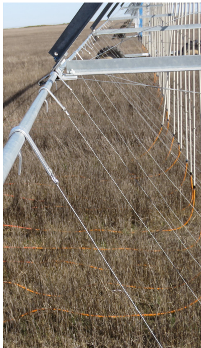
(Above) Using the Truss Rod Assembly Tool, slip truss rod clip onto truss rod and repeat on opposite side.
