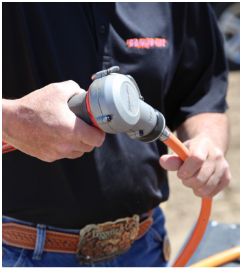
(Above) Use ProPEX tool to expand ends of Dragon-Line flex hose.
