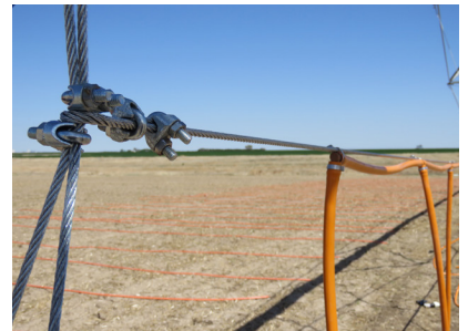
(Above) Low line manifold attaching to tower termination cable w/ minimum of 4' in length remaining to adjust to row spacing.
