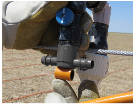
(Above) 1/2" section that is cut out to allow for needed fitting.
