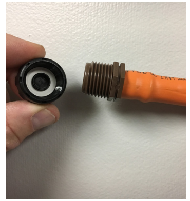
(Above) In the end of the emitter tubing, insert 1/2" MPTxHB 17mm and screw on end cap.
